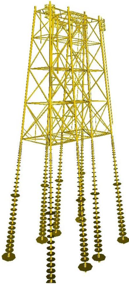
Figure 1 Finite element model of jacket structure.
